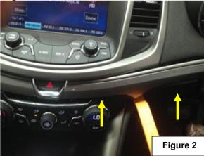
2. Using a 7mm socket remove the 2 screws on both the left and right side(4 screws in total) between the front facia and climate control panel. Refer figure 3 and 4.
